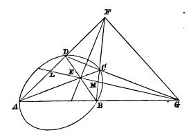
198. DEF. If each of the sides of a triangle be the polar, with regard to a conic, of the opposite angular point, the triangle is said to be *self-conjugate* with regard to the conic.
